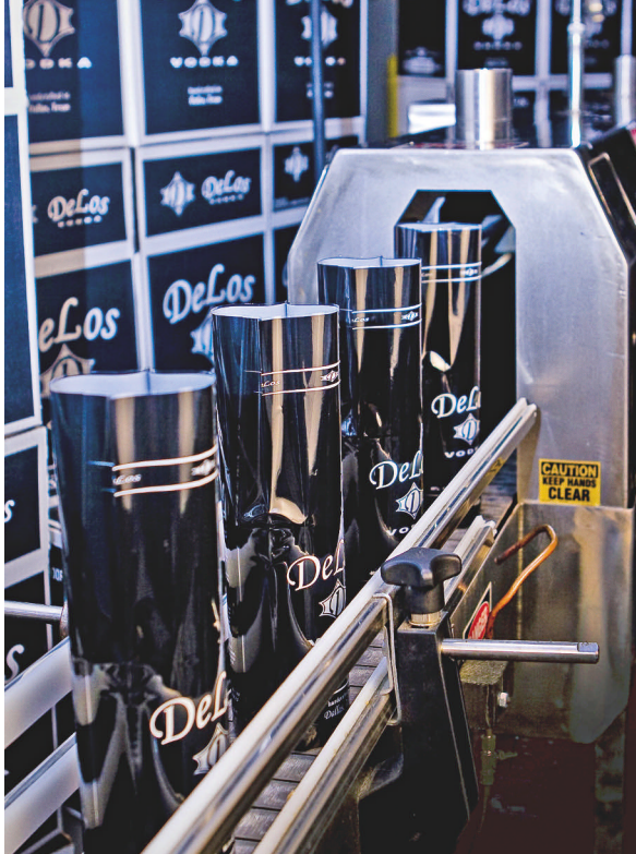
Sleeves are placed over bottles as they enter the steam tunnel, top left. Carlos Guillem, founder of DeLos vodka, fills bottles with his vacuum-distilled vodka, top right. Labeled bottles, bottom right, exit a steam tunnel.
