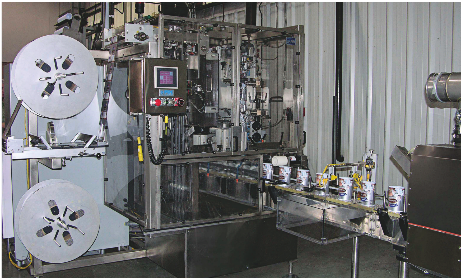
Eastgate Graphics' new shrink labeling system is a patented, mandrel-style machine that operates at speeds up to 300 containers/min. Pictured here are milkshake containers.
